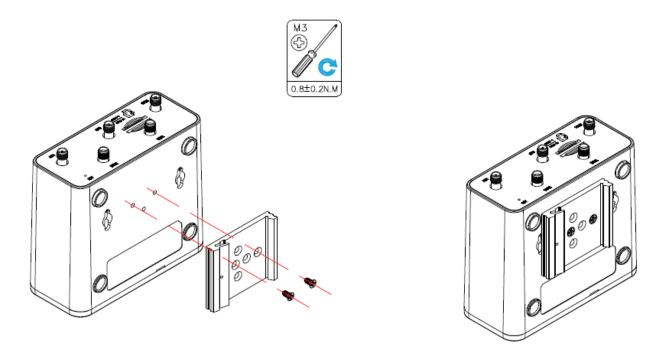
Use 3 pcs of M3\*8 Black cross recessed countersunk head tapping screws to mount the router on the DIN rail, and then hang the DIN rail on the holder. You need to choose a standard holder.
