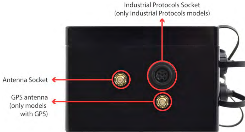
Figure: Antenna side of the enclosure
