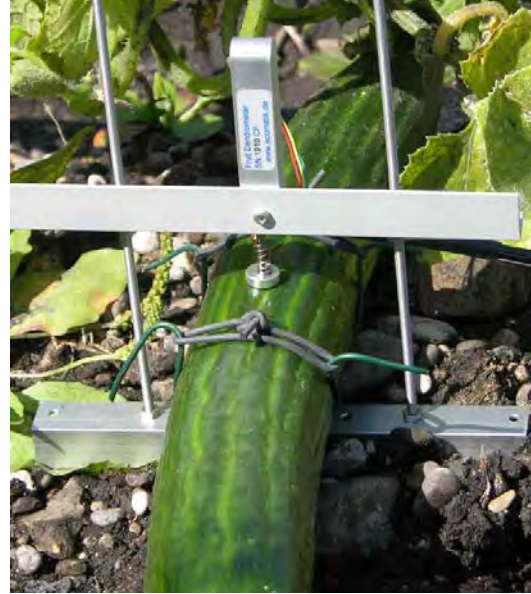
Figure: Ecomatik DC2 sensor (previous version)
