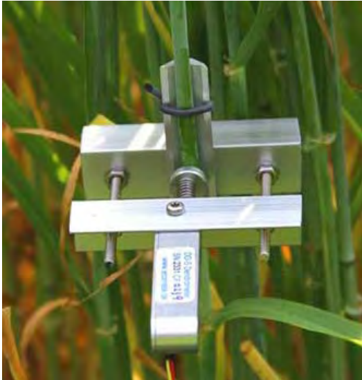
Figure: Ecomatik DD-S sensor (stem)
