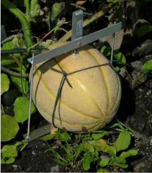
Figure: Ecomatik DC2 sensor (previous version)
