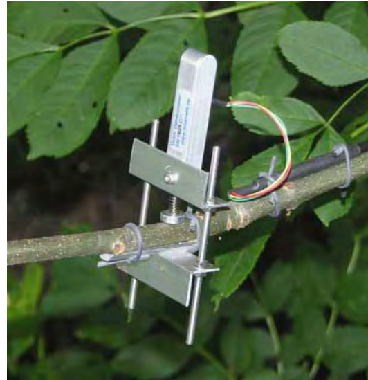
Figure: Ecomatik DD-S sensor (stem)
