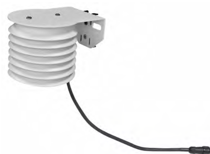
Figure: Vapor pressure, humidity, temperature and pressure in soil and air sensor probe (Decagon VP-4)
