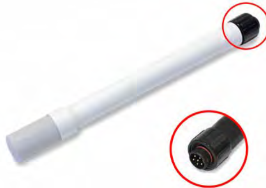
Figure: Temperature, humidity and pressure sensor (Bosch BME280)
