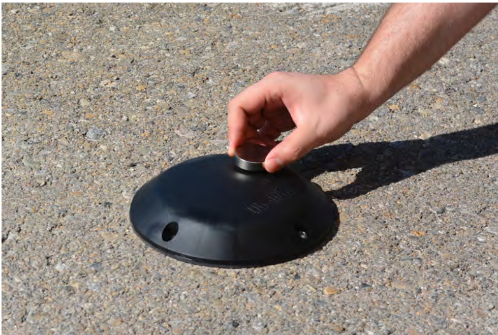
Figure : Using the magnet to start the node
