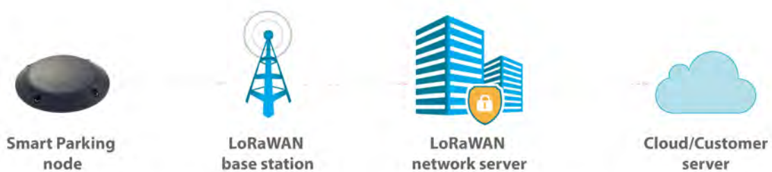
Figure : Simplified Smart Parking network architecture
