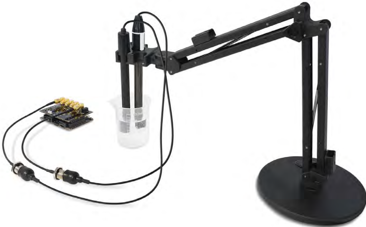
Figure: Calcium Ion ( \text{Ca}^{2+} ) Sensor Probe in 10 mg/L solution
