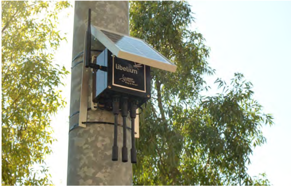
Figure: Wasmote Plug & Sense! powered by an external solar panel
