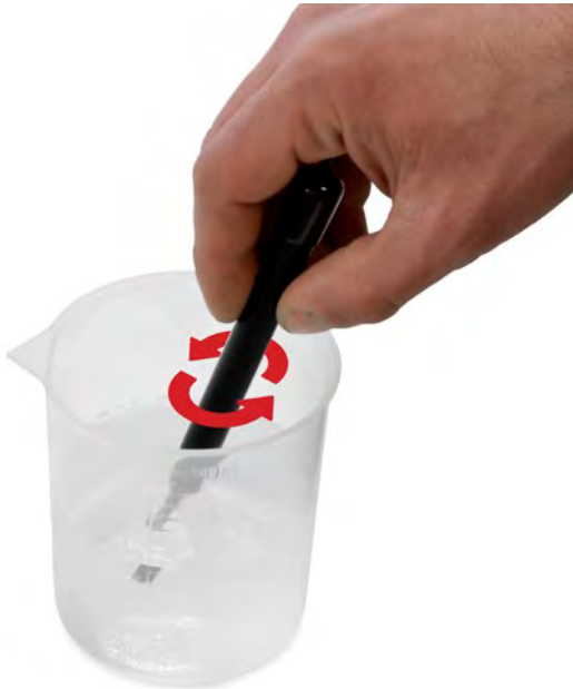
Figure: Cleaning a sensor in deionized water
