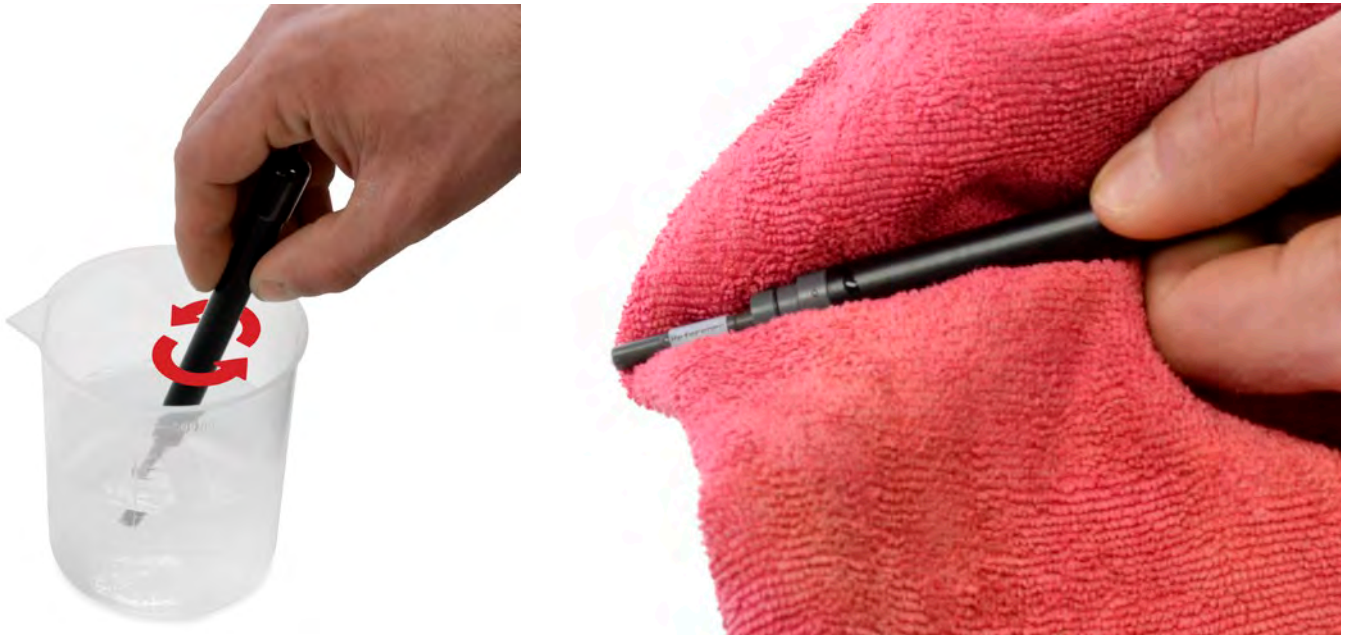
Figure: Cleaning a sensor in deionized water
