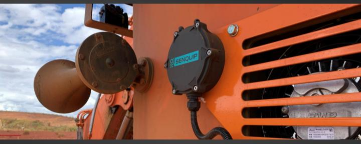
Senquip manufactures rugged, programmable telemetry devices that connect to industrial sensors and system and send the data measured to the Senquip Portal or a server of your choice.
